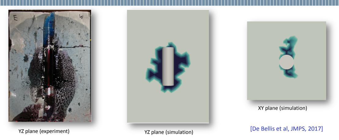
• Missing strength properties estimated from the literature. Assume  $G_c = 100 \text{ N/m}$ ,  $T_c = 5 \text{ MPa}$ , and  $\phi = 31 \text{ degrees}$ . A posteriori damage variable (0 no damage, 1 full damage)
